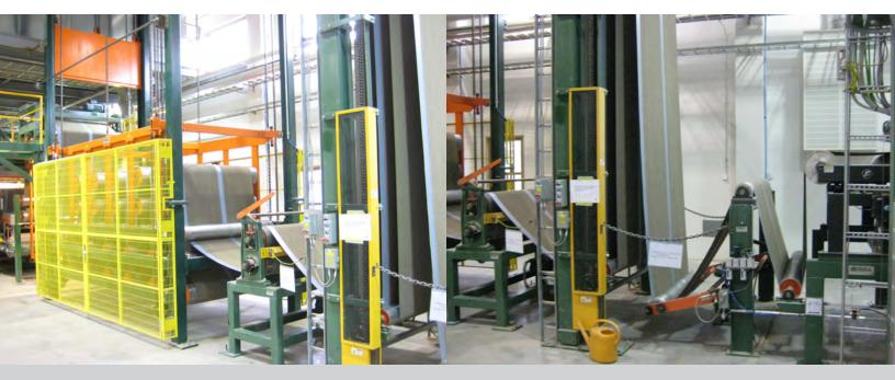
Supercharge the performance of your Roll Winder with a Reichel & Drews servo driven Shock Roll System. Engineered to assure maximum length control at any speed, our driven shock roll system takes out much of the adjustment and guess work normally required when running a wide range of products. Our intuitive user interface and process control allows for seamless product change over with minimal operator input.
