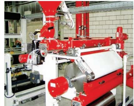
In order to produce sandwich membranes several top coating systems may be arranged in tandem. The thickness of the cover compound layer applied onto the carrier is always determinable and adjustable in a tolerance range of <math><0.1\text{mm}</math>. **System 3000**'s coating system achieves greater material savings because the bituminous membrane can always be produced at the lowest permissible level of thickness. Top side coating is designed as a modular system.
