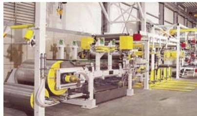
Production line for the production of high-tech bituminous roofing membranes with SBS, APP modified and self-adhesive bitumen compounds (2 top side coating heads, 3 cooling belt coating heads).
